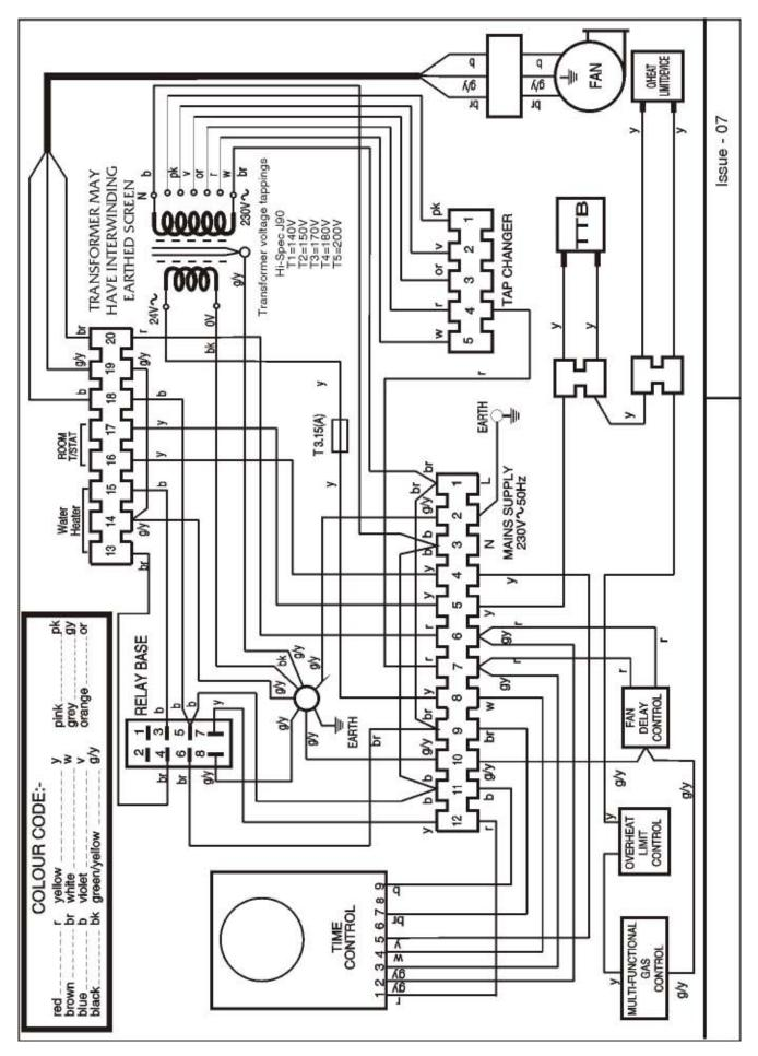
Fig. 5b, Non-MODAIRFLOW CIRCUIT DIAGRAM
