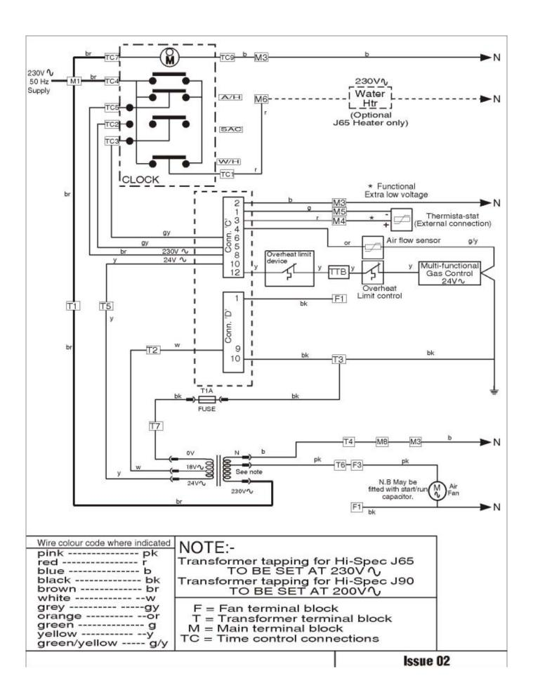
Fig. 6a, MODAIRFLOW FUNCTIONAL DIAGRAM
