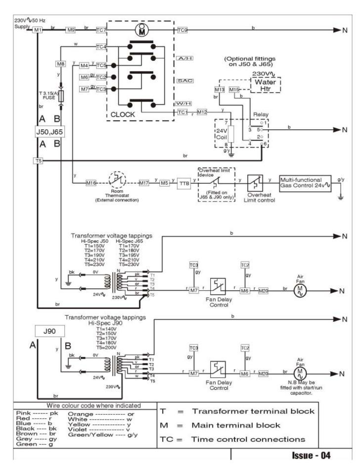
Fig. 6b, non-MODAIRFLOW FUNCTIONAL DIAGRAM
