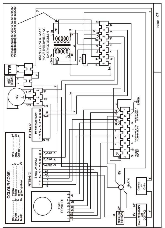
Fig. 5a, MODAIRFLOW CIRCUIT DIAGRAM
